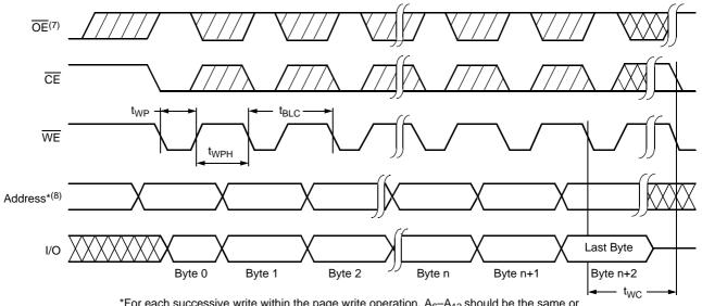
\*For each successive write within the page write operation, A<sub>6</sub>–A<sub>12</sub> should be the same or writes to an unknown address could occur.
