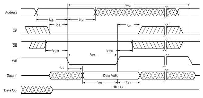
Notes: (5) t<sub>WC</sub> is the minimum cycle time to be allowed from the system perspective unless polling techniques are used. It is the maximum time the device requires to automatically complete the internal write operation.
