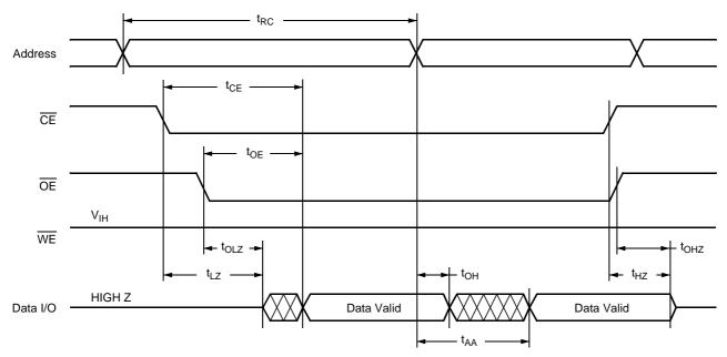
Note: (4) t<sub>LZ</sub> min., t<sub>HZ</sub>, t<sub>OLZ</sub> min., and t<sub>OHZ</sub> are periodically sampled and not 100% tested. t<sub>HZ</sub> max. and t<sub>OHZ</sub> max. are measured from the point when CE or OE return HIGH (whichever occurs first) to the time when the outputs are no longer driven.
