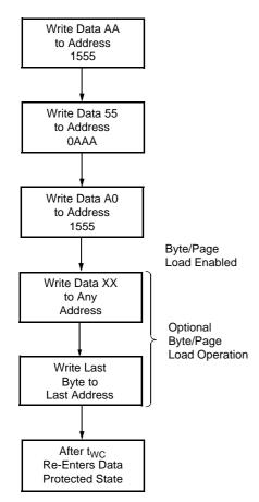
Regardless of whether the device has previously been protected or not, once the software data protection algorithm is used, the X28HC64 will automatically disable further writes unless another command is issued to deactivate it. If no further commands are issued the X28HC64 will be write protected during power-down and after any subsequent power-up.
