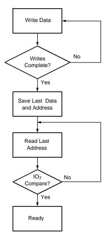
DATA Polling can effectively reduce the time for writing to the X28HC64. The timing diagram in Figure 2 illustrates the sequence of events on the bus. The software flow diagram in Figure 3 illustrates one method of implementing the routine.
